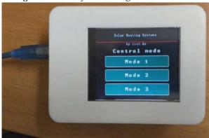
Fig.6. The solar system management controller
