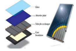
Fig.3. Principal diagram of flat solar collector in parts
