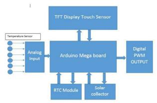
Fig. 5. Block-diagram of managing controller of double circuit solar plant with thermosiphon circulation
