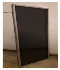
Fig.4. Flat solar collector mockup
